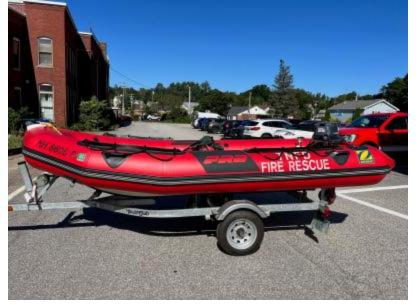
Boat 1 (21B1) is a 2003 Zodiac PRO 420 with a 25 hp Yamaha outboard engine. Boat 1 is used for water rescues in the lakes and ponds and on the rivers.
