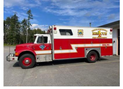
Rescue 1 (21R1) is a 2000 International 4900 with a Marion walk-in rescue body. Rescue 1 has a 20 Kw generator and a complete set of TNT hydraulic rescue tools. Rescue one is used mainly at vehicle collisions
