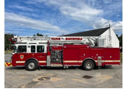
Ladder 1 (21L1) is a 2013 Smeal 75-foot rear mount aerial with a 500 gal tank and a 1500 gpm pump.
