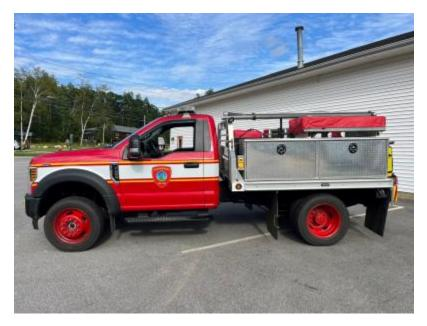
Forestry 1 (21F1) is a 2017 Ford F450 4X4 with a CTE forestry skid unit with a pump and 250 gal tank. This truck is equipped to respond to forest and brush fires.
