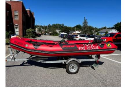
Boat 1 (21B1) is a 2003 Zodiac PRO 420 with a 25 hp Yamaha outboard engine. Boat 1 is used for water rescues in the lakes and ponds and on the rivers.
