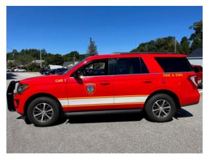
Car 1 (21C1) is a 2019 Ford Expedition. It is equipped as a command car and carries basic first aid materials, a semiautomatic defibrillator, and firefighting personal protective gear.
