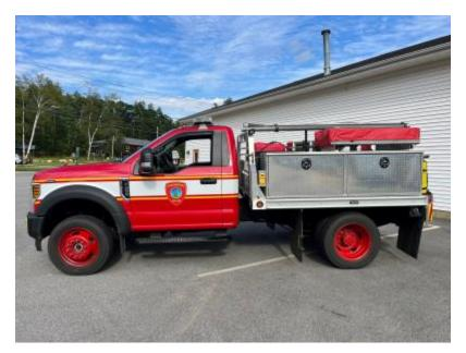
Forestry 1 (21F1) is a 2017 Ford F450 4X4 with a CTE forestry skid unit with a pump and 250 gal tank. This truck is equipped to respond to forest and brush fires.
